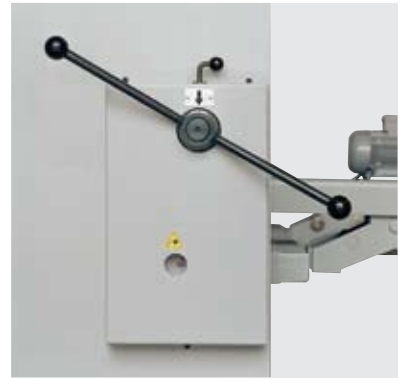
Manuel sentil ayar sistemi Manual blade gap adjustment
